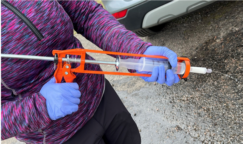
Firing the sealant gun to filter sample water.
