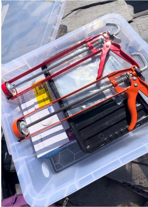
Example of field box containing all consumables, gloves and sealant guns. Note the secondary box (black lid) for sensitive consumables.
