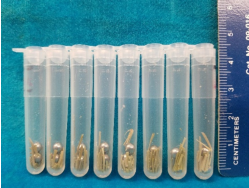
Figure 3. Grinding set-up for dry material.
