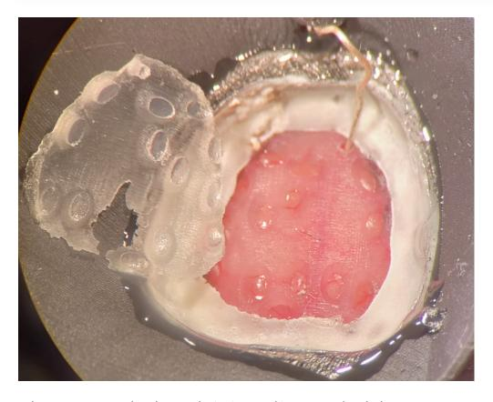
Elastomer removed and ground wire inserted into grounding hole.
