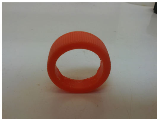
Fig 2: 50 mL falcon tube lid with the centre of the lid top removed.
