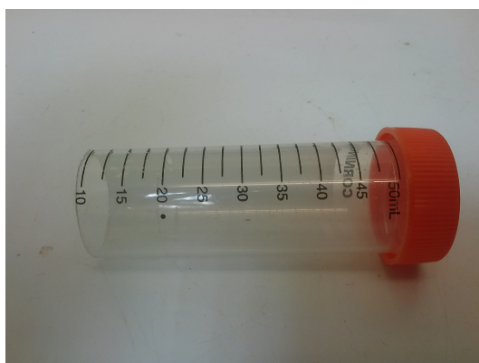
Fig 1: 50 mL falcon tube with the bottom ~2 inches removed.
