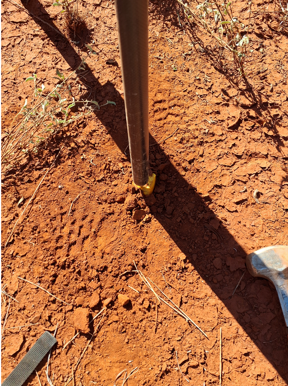
Capped ground stake used as central position for D-RTK2.
