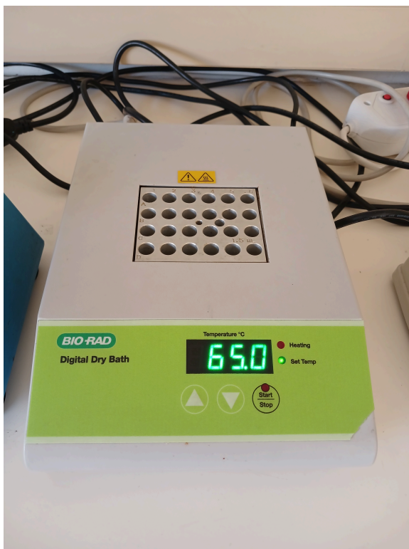
Heating block set to 65 degrees Celsius.
