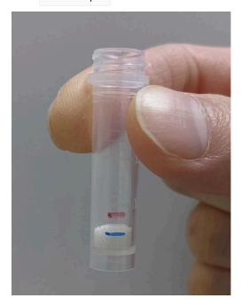
2 Add  $\perp$  200  $\mu$ L of **1 mm beads** to 2mL screw tube
