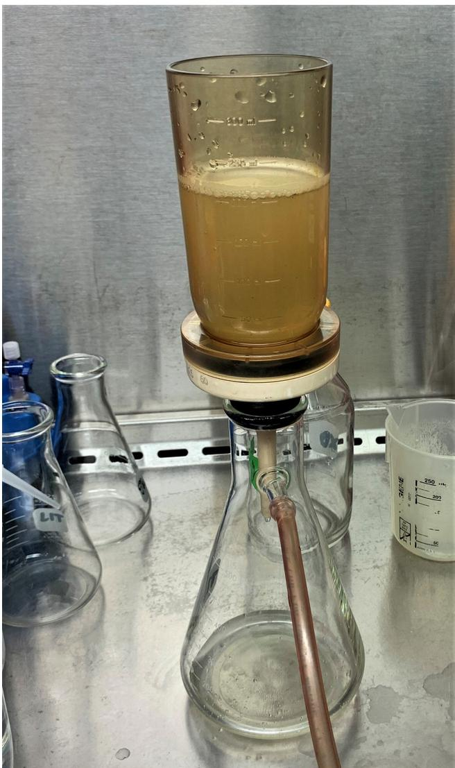
Wastewater filtering through a 5-um PVDF filter in a Pall filter holder.
