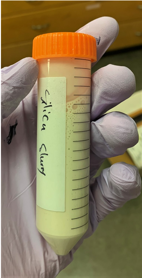
"Milk of Silica" suspension (1g silicon dioxide/mL water)
