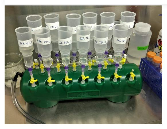
Passing lysed & filtered samples through Zymo III-P columns for direct RNA capture.
