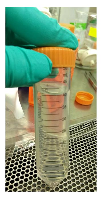
Filtered sample before ethanol addition. Filtrate should be semi-clear.
