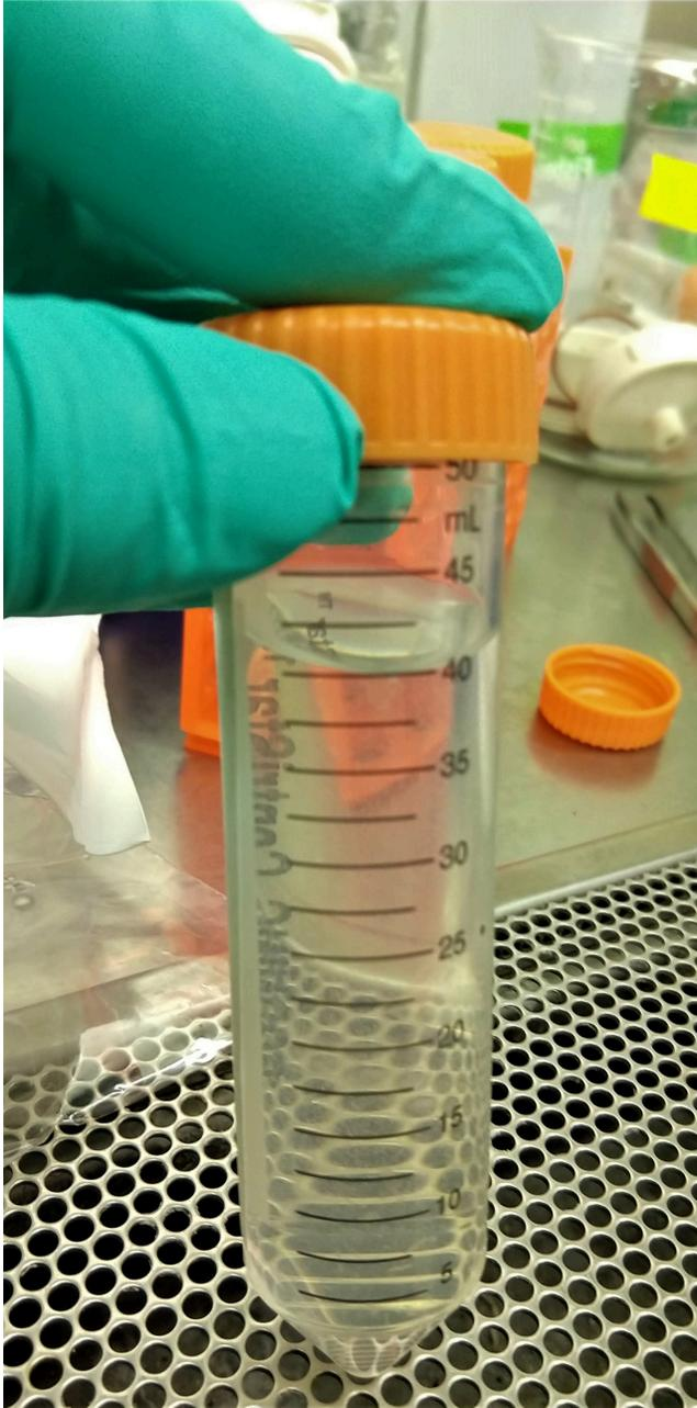
Filtered sample before ethanol addition. Filtrate should be semi-clear.
