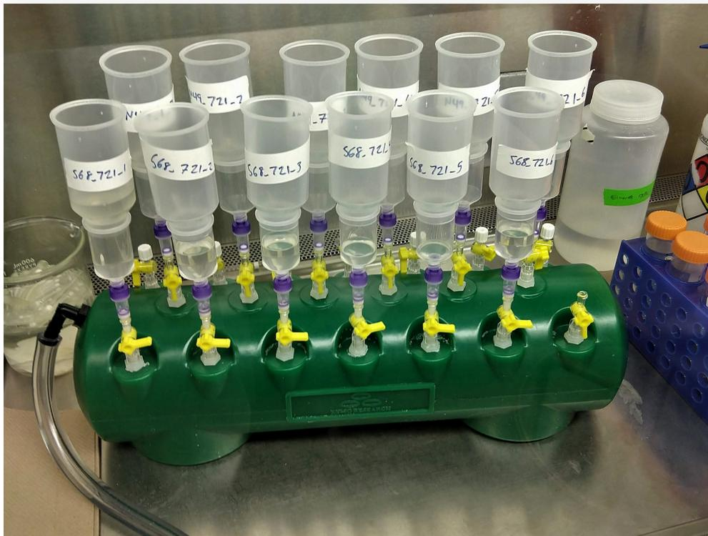
Passing lysed & filtered samples through Zymo III-P columns for direct RNA capture.
