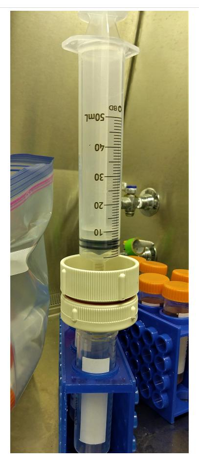
Syringe filter setup: Wastewater is filtered through a 47-mm reusable filter membrane holder.
