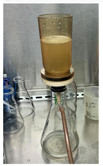
Wastewater filtering through a 5-um PVDF filter in a Pall filter holder.
