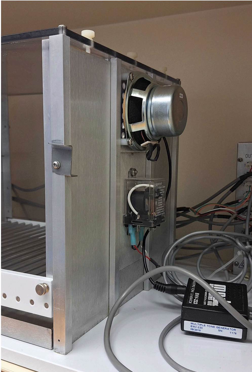
Picture 1. Chamber back panel from the outside showing the central placement of the clicker and speaker, with the tone generator box to the right.
