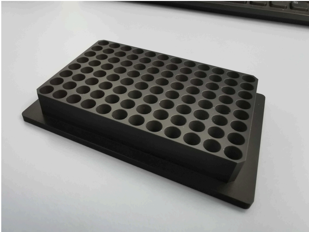
Plate adapter for 96 well PCR plates for CPAC, supplier: Hamilton company.
