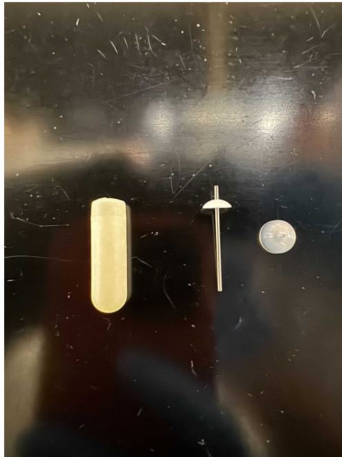
Figure 2. Components of Osmotic Pump. On the left is the storage component of the osmotic pump. In the middle is the flow moderator. On the right is the cap. This is how they will be referred to in future steps.
