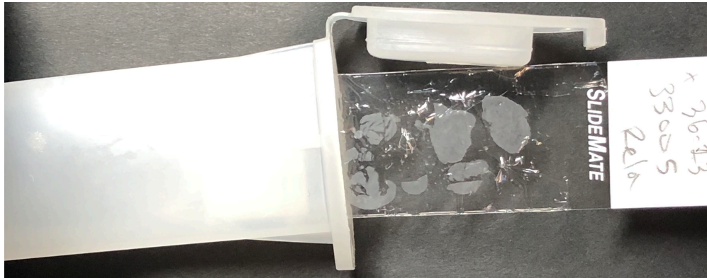
Figure 2: A small slide holder will hold two plastic film-wrapped slides without touching or disturbing the wrap. Closing the top will allow for long incubations without drying out. For small tissue sections (e.g. 1 cm 2 ), using small plastic wrap squares that cover the sample but do not wrap around the slide will require proportionally less volume, saving on reagent costs.
