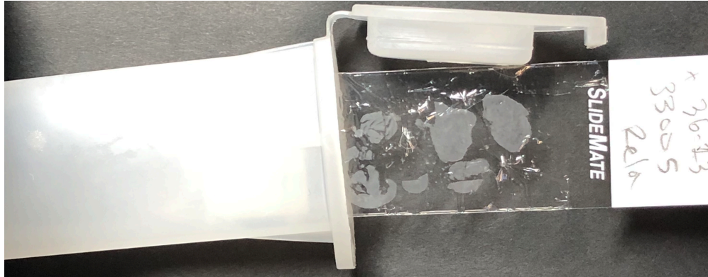
Figure 2: A small slide holder will hold two plastic film-wrapped slides without touching or disturbing the wrap. Closing the top will allow for long incubations without drying out.
