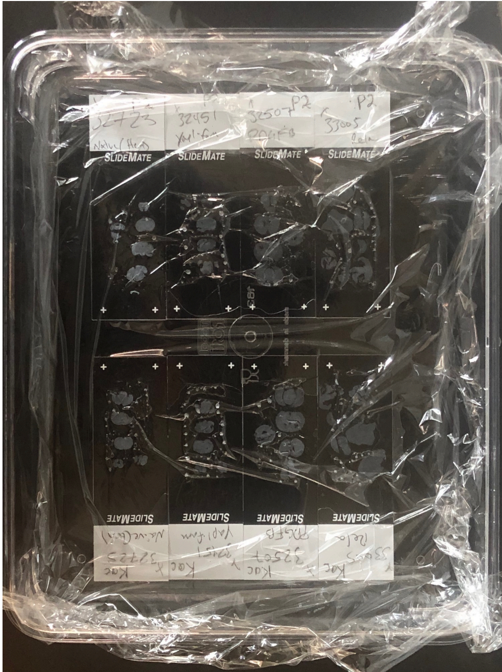
Figure 3: Optional setup for incubating multiple slides with the same solution.
