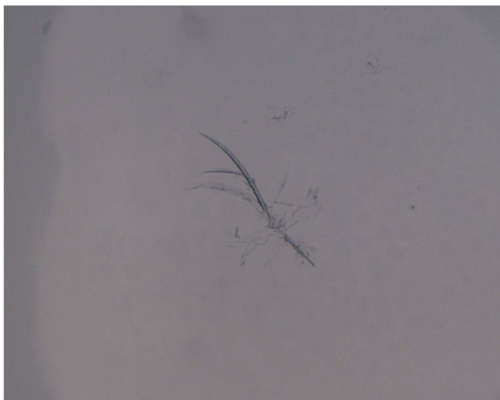
Fig. 1 Microscopic image of “ugly” Clusterin mutant TL1 crystals in Classics condition H3. The overall image dimensions are approximate 0.75 x 1 mm.
