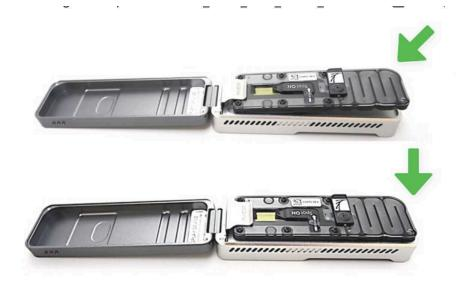
16 Slide the flow cell priming port cover clockwise to open the priming port.
