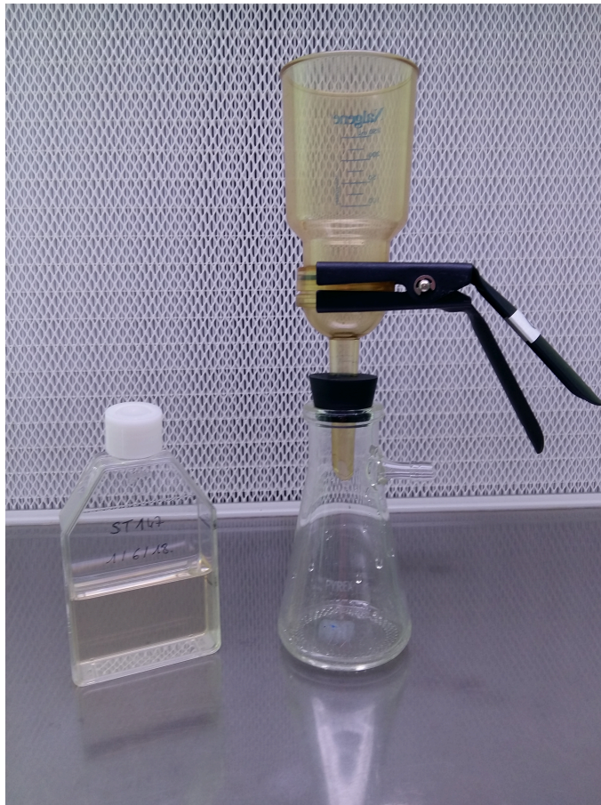
Picture : Filtration on Nylon 10 \mu filter with a Nalgen filtration system
