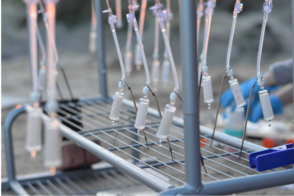
Close-up view of the Sterivex filters secured with small bungee cords (Photo Credit: Callie Chappell)
