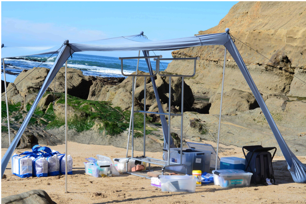
Example field set-up with clothes rack and shade structure (Photo Credit: Callie Chappell)
