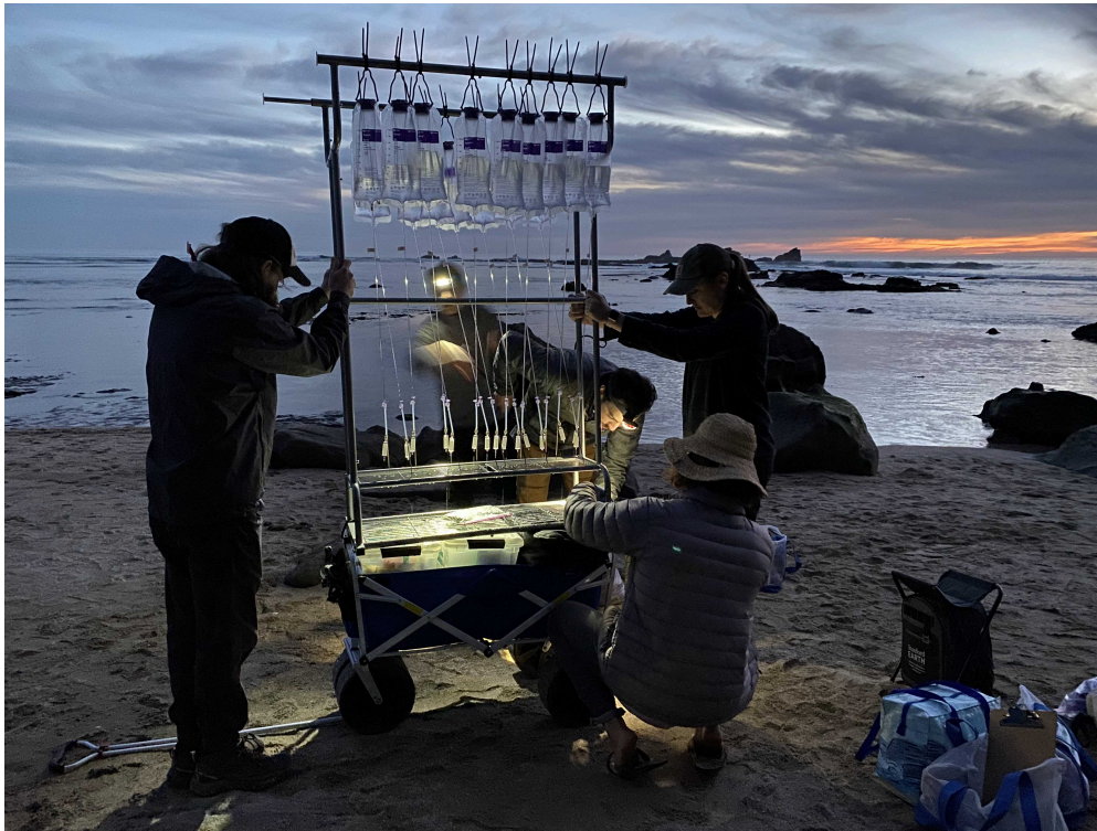
Example of mobile filtration set-up (Photo Credit: Callie Chappell)
