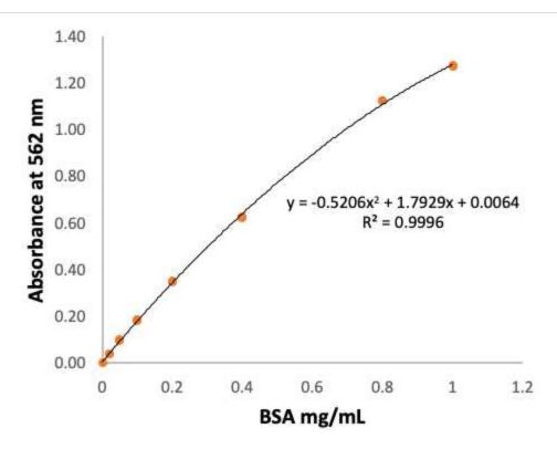
For the calculation convenience, plot BSA concentration (Conc) versus Corrected absorbance (Abs) to obtain a standard curve as following:  $Conc_mg/mL = a \times Abs^2 + b \times Abs + c$
