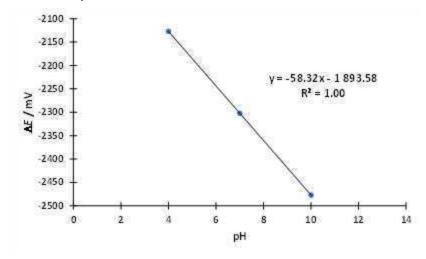
Calibration graph of a glass electrode half-cell.
