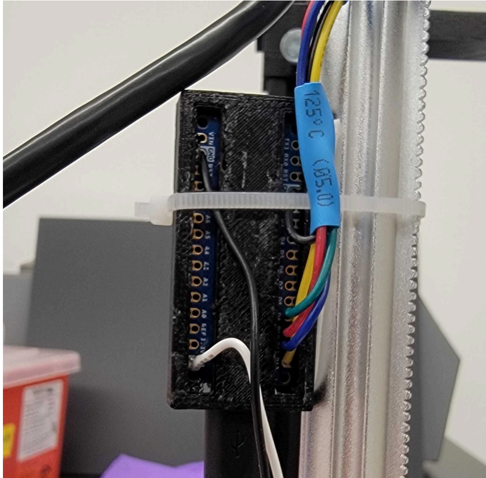
Arduino Nano Every wired together in its case
