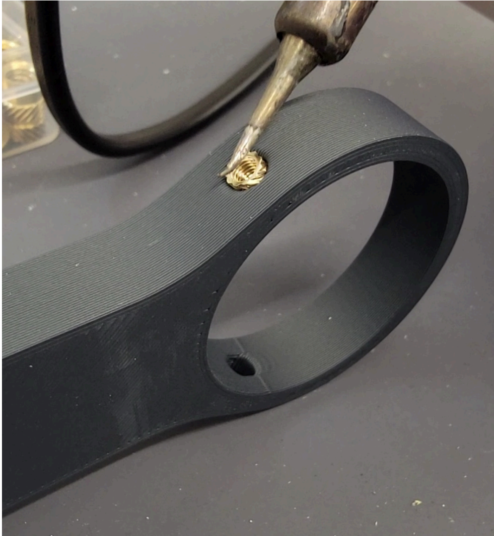
Adding a 4 mm M3 threaded insert to the camera holder
