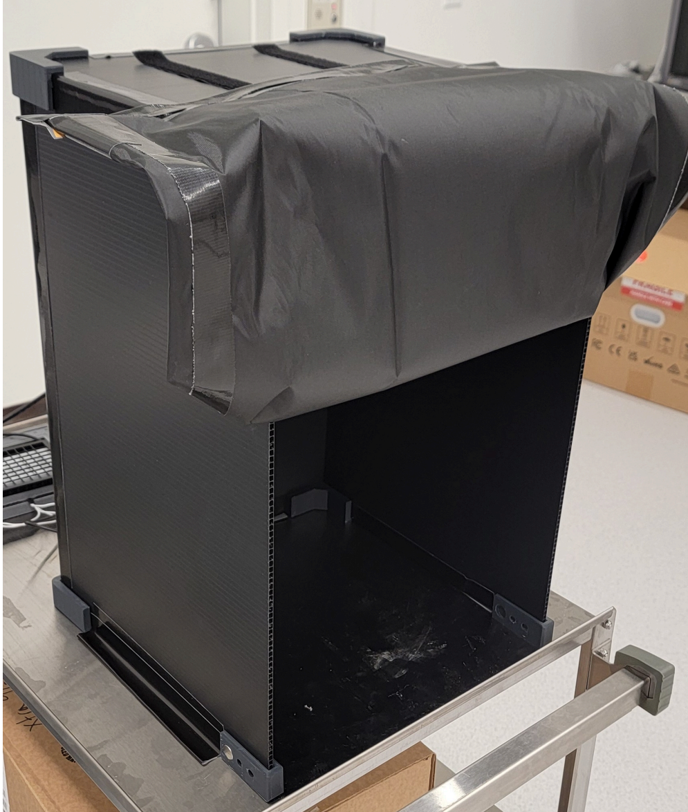
A phenotype-o-mat dark box made with 3D-printed brackets
