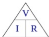
Figure 17. Illustration of the relationship between voltage (V; Volts), current (I; amps) and resistance (R; ohms), according to Ohm's Law.
