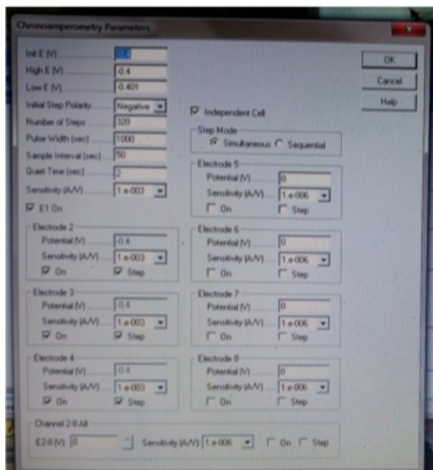
Figure 6a. Software settings for chronoamperometry run. These set the machine going for the longest it can (~3 days) but it is HIGHLY RECOMMENDED you stop, save and re-start once a day (except weekends, obviously). Just in case
