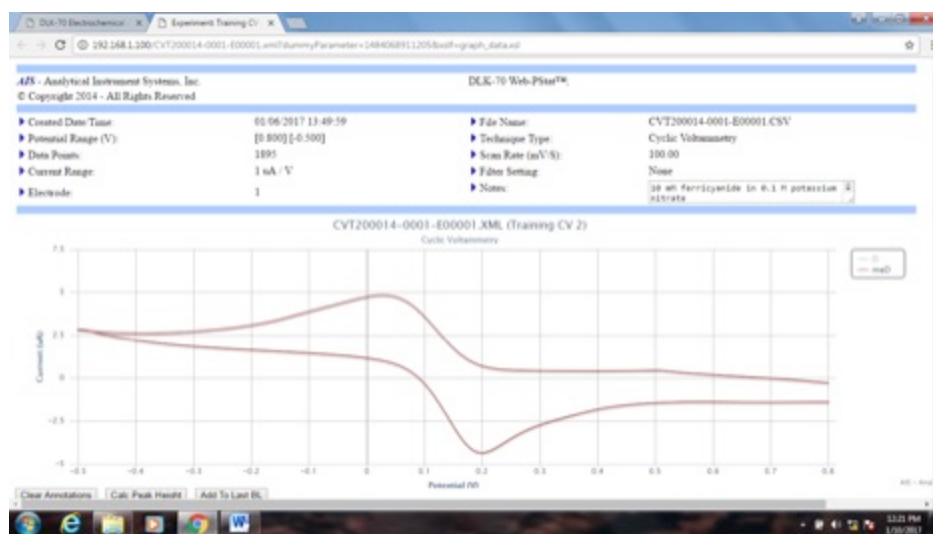
Figure 13. Cyclic voltammograms (a CV program with Test Solution) showing an extended tail
