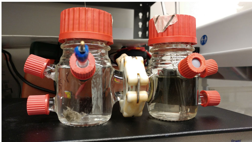
Figure 2a. Schematic of cells complete and ready to go. Note, gas exchange ports are not included in working cell for this configuration. RE = reference electrode, WE=Working electrode (ITO glass) and CE= counter electrode (Carbon cloth). Filters are 25 mm 0.2 \mu m mesh Whatman filters in autoclavable filter holders. PEM = pre-soaked Nafion 117 proton exchange membrane and gasket, secured with knuckle clamp. Right cell is counter, left cell is working. See “day of” instructions for detailed information about placement.
