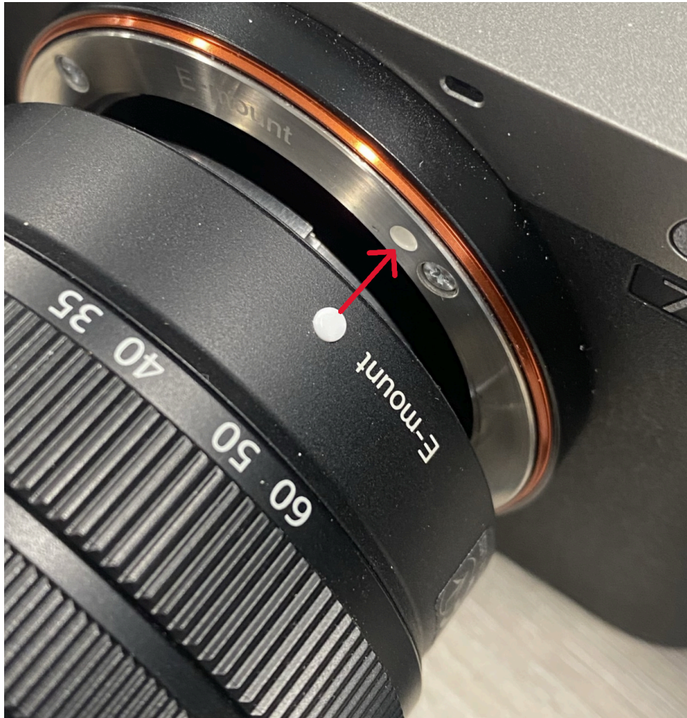
Aligning the white dot on the lens with the white dot on the camera.
