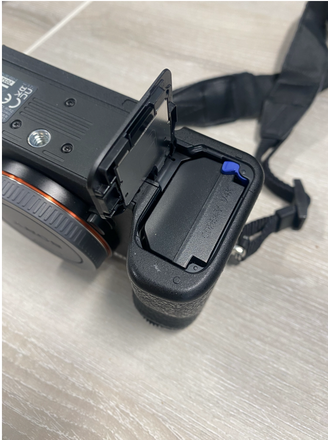
Battery Compartment - Battery in place
