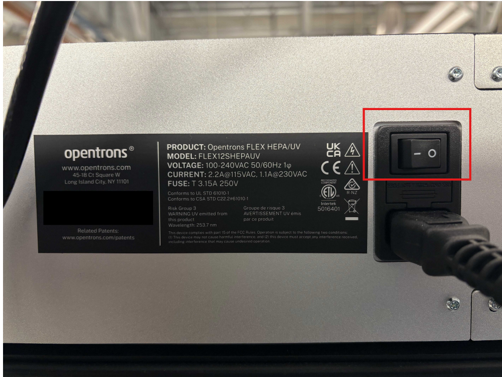
Figure 3. HEPA/UV module power panel with the power switch outlined in red.
