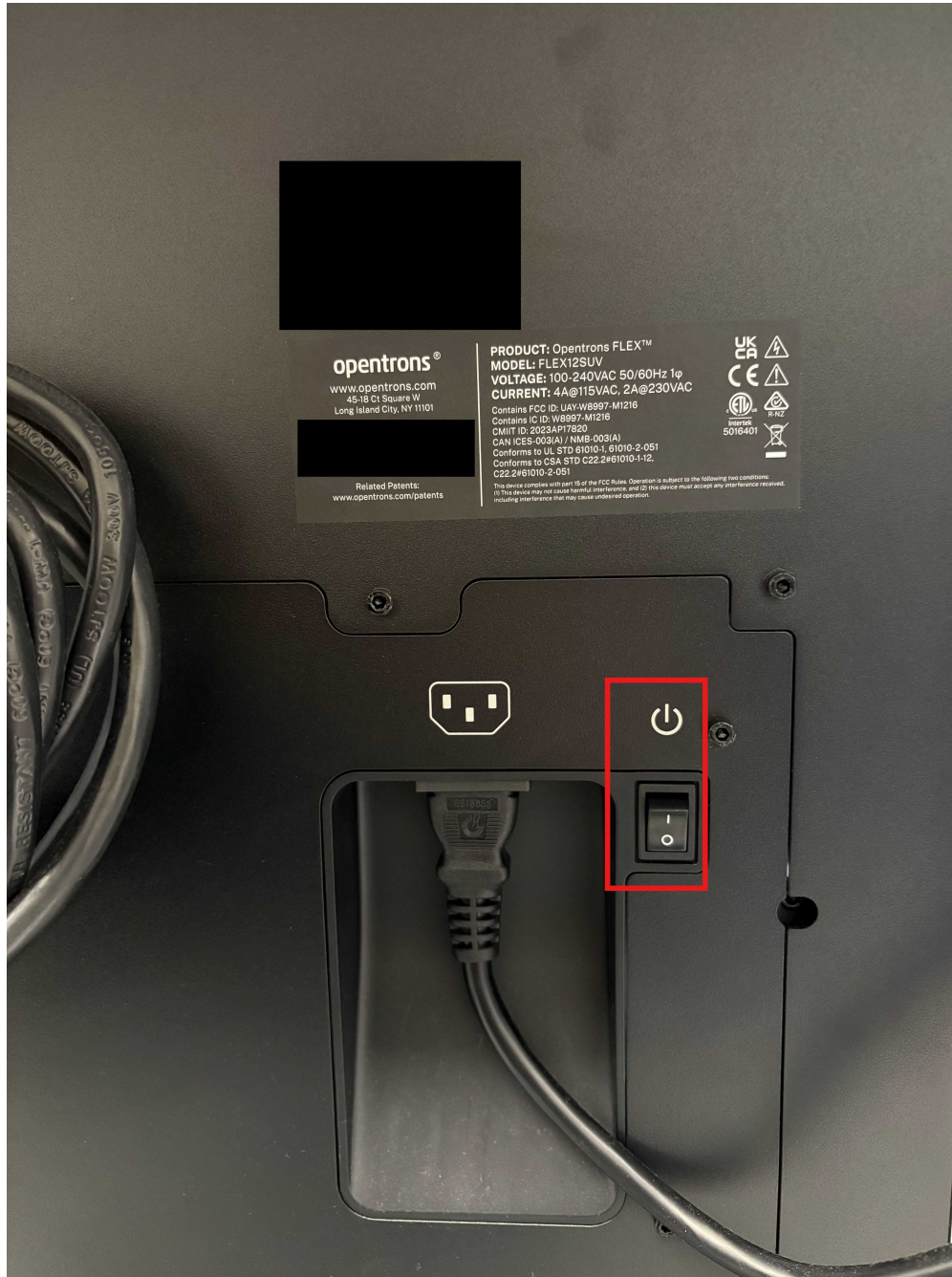
Figure 2. Opentrons Flex power panel with the power switch outlined in red.
