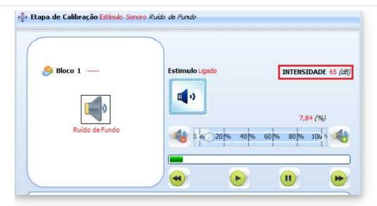
Adjust the intensity of the sound manually in the percentage bar and press play. Check the decibel meter inside the equipment to see if the desired range is shown. If it is, click on the next button. You can adjust the sound range with the buttons at the beginning and the end of the percentage bar, or move it freely with the mouse by sliding the bar;
