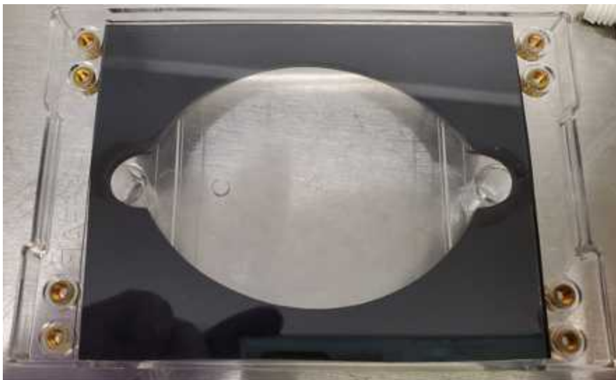
Fig. 5: Glass slide placed on the silicone gasket
