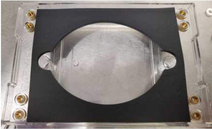
Fig. 4: Upside-down EcoFAB 2.0 base with silicone gasket
