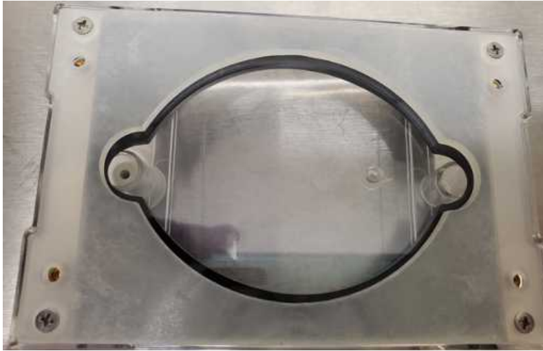
Fig. 9: EcoFAB 2.0 with screws fully tightened
