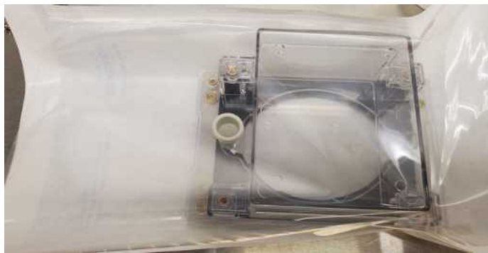
Fig. 8: EcoFAB 2.0 in an autoclave bag
