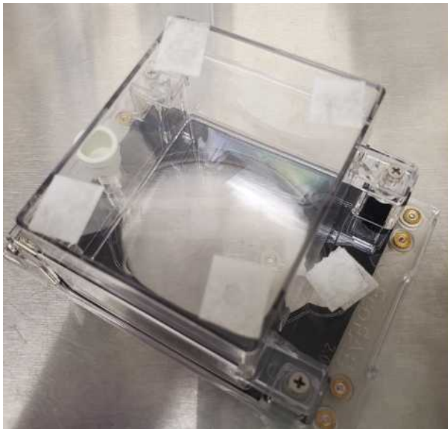
Fig. 10: Micropore tape covering the chamber vents and the sampling port
