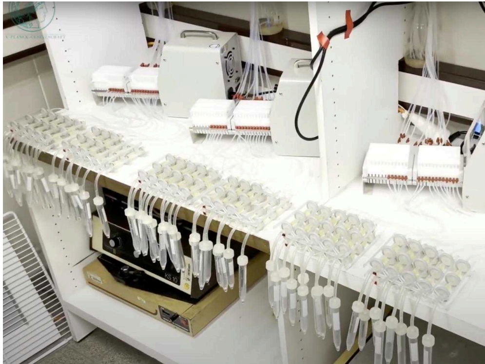
Figure 6: Example of a final MetaFlowTrain setup. This setup includes trains consisting of two microchambers, with four pumps running in parallel, resulting in 72 samples. Note that the MetaFlowTrain racks can be stacked to save space
