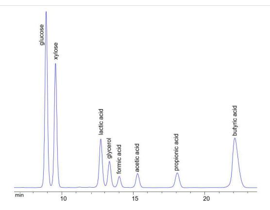
Elution order for analytes included in the commercially available 'Carboxylic Acid Standard Kit' seen in 'Materials'.
