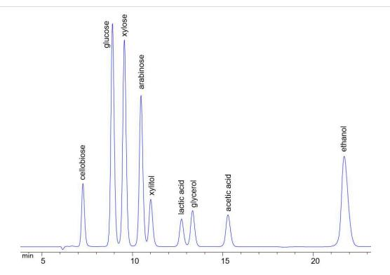
Elution order for analytes included in the commercially available 'Coferm Standard Kit' seen in 'Materials'.
