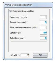
Latency = 60ses: 1min for acclimatization before the recording. Record time= 5min: We record 5min for each mouse.
