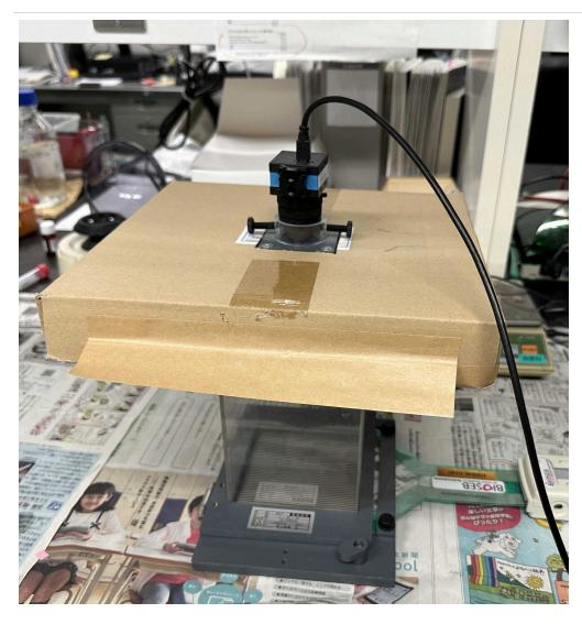
We made the apparatus a hat to reduce the reflection of room light.
