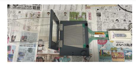
Embed the sensor in the floor of the chamber.
