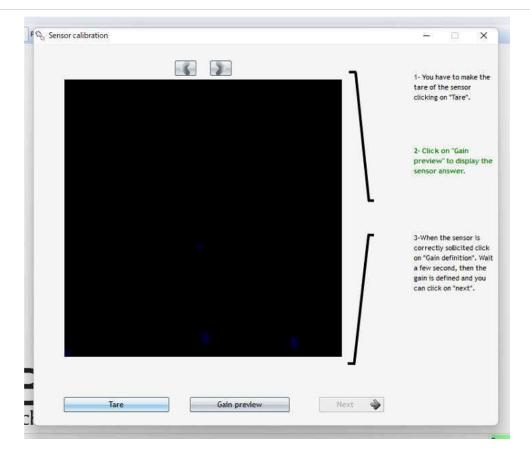
Click "Gain preview", and apply the calibration weight (3000g) indirectly on the sensor.
