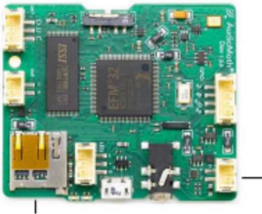
Figure 1. Backside of the AudioMoth. The battery terminal is shown in the bottom-right corner (image provided by WildMon, 2024).
