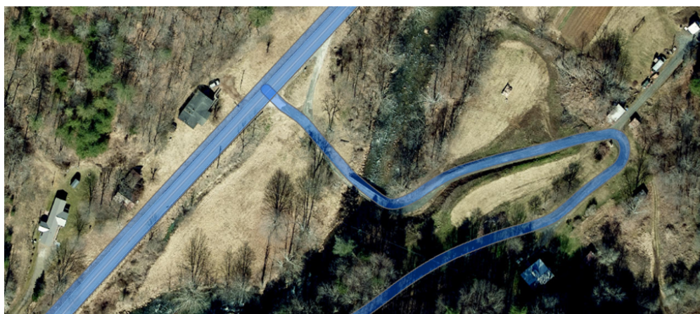
Figure 5 – Road center lines buffered variable amounts according to route category (Table 3). Each buffered road was assigned a material ID, converted to a raster, and added to the materials raster.
