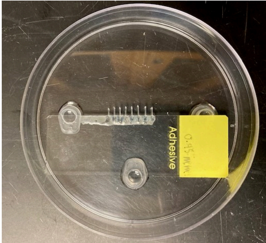
Figure 5. Slide holder made of a petri dish and microcentrifuge tube lids holding the grafting slide in place.
