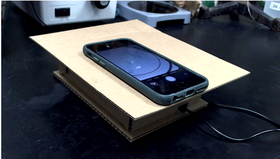
Figure 12. phone camera aligned with lens and centered on sample.
