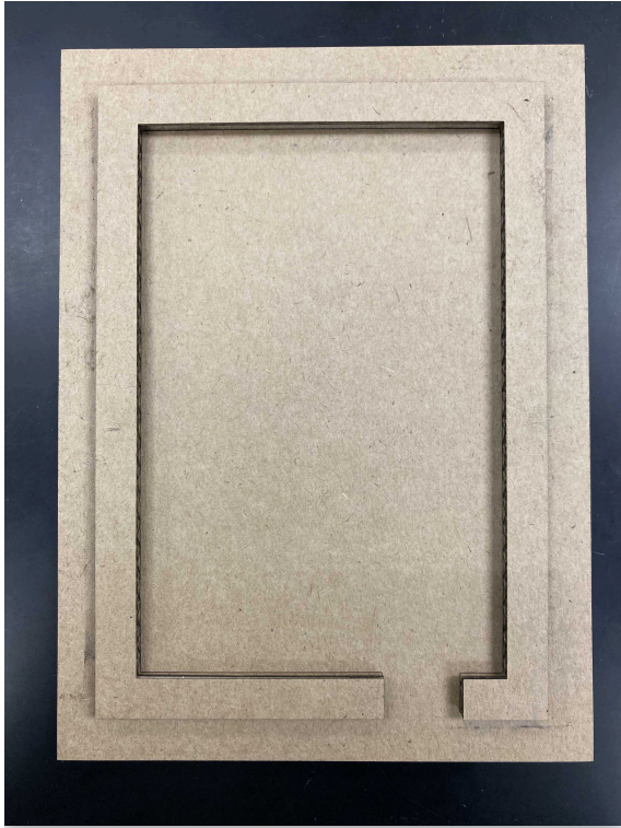
Figure 2. Light panel support attached to base.
