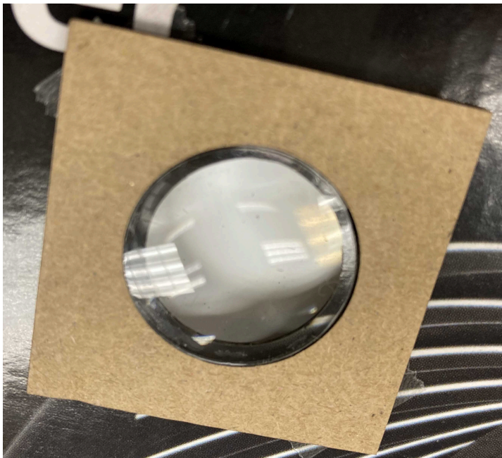
Figure 5. lens inserted in the spacer.
