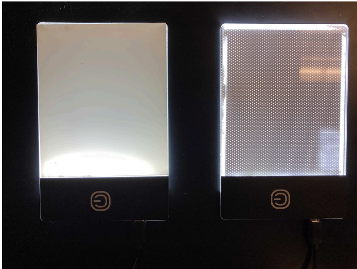
Figure 8. Left: light panel with vinyl sheet attached. Right: light panel without vinyl sheet.
