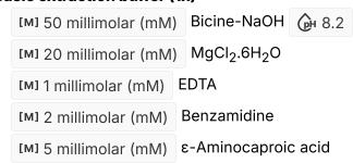
■ Dissolve in ultrapure  $H_2O$ ; adjust pH to 8.2 with NaOH; degas the solution bubbling with nitrogen (5 min/100 mL), then add:
