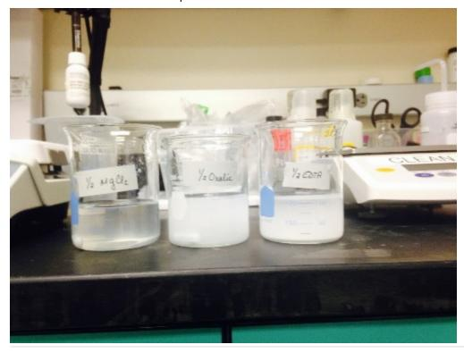
Note the  $\frac{1}{2}$  MgCl<sub>2</sub> beaker on the left is the most clear but still a little cloudy. The  $\frac{1}{2}$  Oxalic acid is very cloudy, but can still see the stir bar at the bottom. The 1/2 EDTA has an obvious white precipitate at the bottom that will not go back into solution. This picture is about 2 hr after the final pH and QS to 100ml. Stirring does not make the cloudiness or precipitates go into solution.
